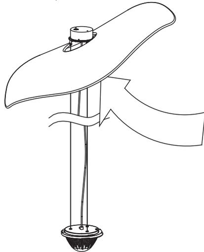
**B** Connect to the circuit according to the connection table. If necessary cut the cable and reconnect as it was; you will need to release the cable by loosening the 3 threaded rod. Reconnect as it was; you will need to release the cable by loosening the rod 3, tighten it to lock the cable.
