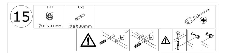
Connect No. 12 with No. 17 plate using wooden dowel (C) and turn cam lock (B) in No. 12 plate clockwise to tighten as shown.
