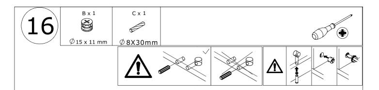
Attach No. 11 plate to No. 15 wooden doweCand turn cam and turn cam lock (B)
