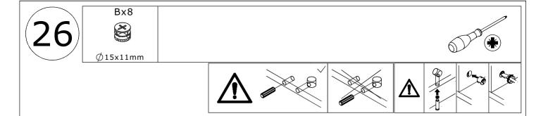
Connect No. 27 late with No . 29 a nd No. 30, turn cam lock (B) in No. 29 30 plate clockwise to tighten as shown.
