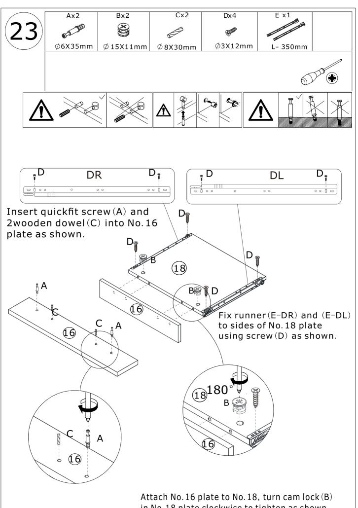
Attach No. 16 plate to No. 18, turn cam lock (B) in No. 18 plate clockwise to tighten as shown.
