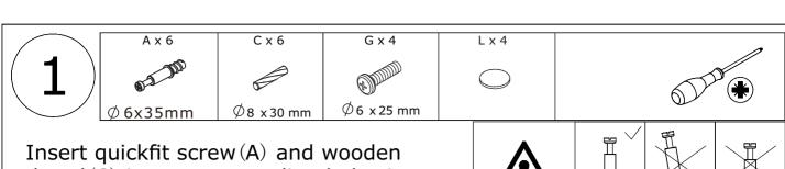
Insert quickfit screw (A) and wooden dowel (C) into corresponding holes in No. 6 plate as shown.
