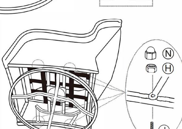
Step 4: Tip chair over with one side on the ground. Attach U-shape fitting to arms with with 4pcs bolts (J), 4pcs nuts (H) and 4pcs plastic cap(N). Verify the alignment and adjust, now fully tighten all the bolts unsing Hex Wrench (K) and Wrench (L) Put seat cushion and back pillows on.
