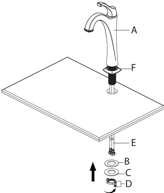
Before installation, ensure that the flange (F) is placed on the bottom of the faucet assembly (A). Place faucet (A) through the 1-3/8" holes in countertop . Secure the faucet (A) to the countertop using the plastic washer (B), metal washer (C) and nut & screws (D) provided. Hand tighten the nut onto the end valve shank. Lock the nut into position by tightening the screws (D) with a phillips screwdriver.
