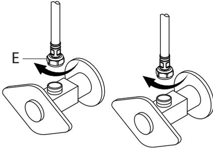
Attach waterlines(E) to angle stops and tighten until snug. Turn on angles stops and check for leaks (DO NOT TURN FAUCET ON)
