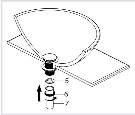
Slide the nut (6) over the tail pipe (7). Place the washer (5) into the nut and tighten. Do not overtighten.
