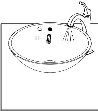
After installing faucet, remove aerator (G) with included aerator key (H). Turn water on for 30 seconds to remove any debris. Reassemble aerator (G).
