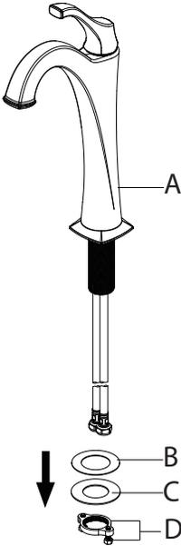
Shut off the water supply. Remove the old faucet. Clean the mounting surface. Remove the plastic washer (B), metal washer (C) and nut & screws (D) from the faucet (A).
