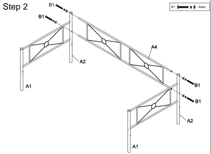
Assemble Back Frame A4 to Rear Legs A2 using Bolts B1 with spring washers and flat washers. (NOTE: Please do not tighten Bolts B1 until Step 5.)
