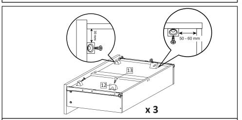
**STEP4**: Insert the Screw M3.5x15.5mm (HW13) and wedge (HW12) into the bottom of the drawer according to the picture.
