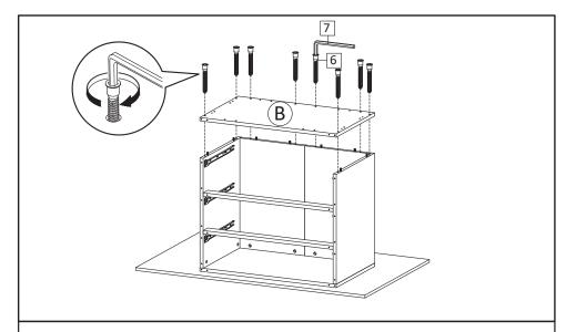
**STEP10**: Insert Bottom Board (B), secure with Screw M7x50mm (HW6), tighten screws using Allen Key (HW7).
