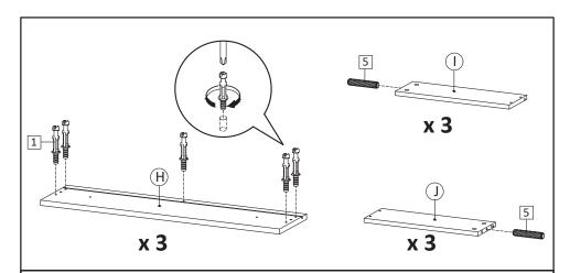
**STEP1**: Insert Cambolt (HW1) into Front Drawer (H). Insert Dowel Small (HW5) into Side Drawers ( I & J )
