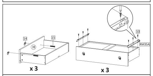
**STEP3**: Use Screw M4x20mm (HW15) to attach Handle (HW14) to the Front Drawer.
