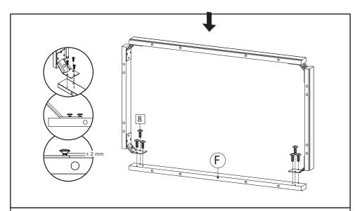
**STEP13**: Combine components from step 12 with remaining Bottom skirt 1 (F), using M4.5x12.5mm (HW8). Do not overtight screw yet, leave around 2mm gap.
