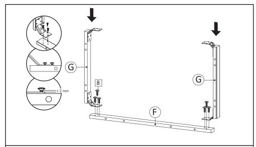
**STEP12**: Combine the Bottom Skirt 2 from step 11 with Bottom skirt 1 (F), using Screw M4.5x12.5mm (HW8). Do not overtight screw yet, leave around 2mm gap.
