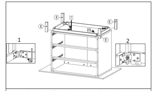
**STEP16**: Place the Leg (E) on the center corner brace and insert the screw M6x25mm (HW20) with Allen Key (HW7) into the leg, then tighten all the screws.
