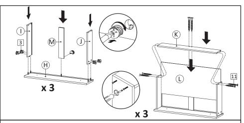
**STEP2**: Combine Side Drawers (I & J) and Support Drawer (M) into Front Drawer (H) then tighten camlock (HW3) using screwdriver. Insert Bottom Drawer (L) with laminated face facing upward then put Back Drawer (K) and secure with Screw M8x39mm (HW11).
