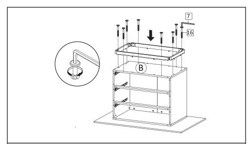
**STEP15**: Bring the assembled bottom skirt and insert into Bottom Board of the chest drawer. Secure the bottom skirt by inserting Screw M6.4x53mm (HW16) and Allen Key (HW7).
