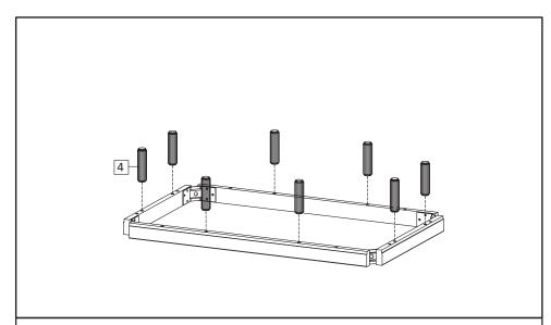
**STEP14**: Insert Dowel Big (HW4) into assembled Bottom skirt from previous step.
