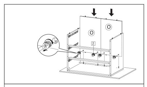
**STEP9**: Insert Back Board (O) Secure with Camlock Big (HW2) and tighten it using screwdriver.
