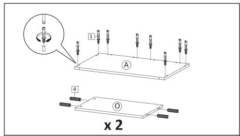
STEP5: Insert Cambolt (HW1) into Top Board. Insert Dowel Big (HW4) into Back Board (O)
