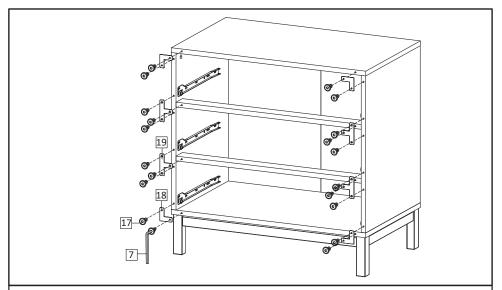
**STEP17**: Bring the chest drawer upright. Install Plat L (HW18), Plat T(HW19) into the provided holes at front edges of the media stand. Secure with screw M 6.4x14mm (HW17),tighten using Allen Key (HW7).
