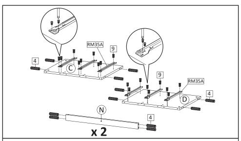
**STEP6**: Insert Dowel Big (HW4) into Side Board Left (C), Side Board Right (D) and Support Board (N). Continue with securing part of the metal runner (HW RM35A) into position as the above image, using screw M6x10.5mm (HW9).
