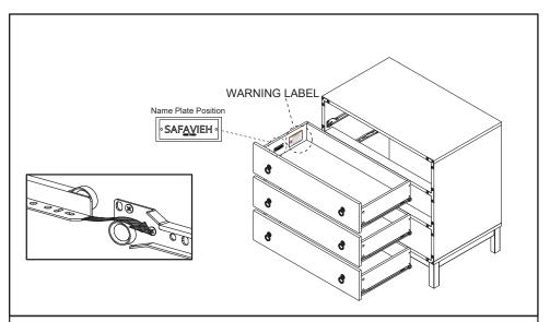
**STEP18**: Hold the sides of drawer, position the wheel of rail at drawer back and the wheel of rail at side boards, according to the image. Slide in the drawers one by one into the chest drawer.
