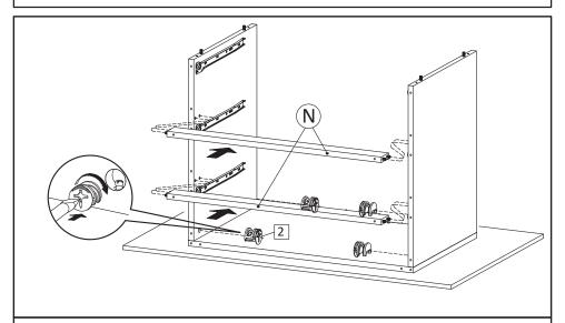
**STEP8**: Attach Support Board (N) Between Side Board Left (C) and Side Board Right (D).
