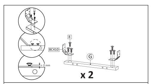
**STEP11**: Now let's combine the bottom skirt. Start with installing Corner Brace (HW BC410) into Bottom Skirt 2 (G) using Screw M4.5x12.5mm (HW8). Do not overtight screw yet, leave around 2mm gap.
