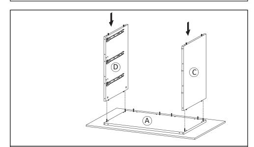
**STEP7**: Attach Side Board Left (C) and Side Board Right (D) into Top Board (A).
