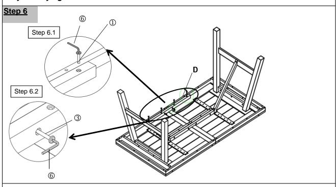
Position Side Support Bar(D) as shown in picture above.
