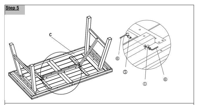
Position Middle Support Bar(C) as shown in picture above. Insert 4 Long Bolts(①) and Sleeve nut (⑤) through the mounting positions and affix the Middle Support Bar(C) to Table(A) using the Allen Key (⑥) **Only loosely tighten the Bolts.**
