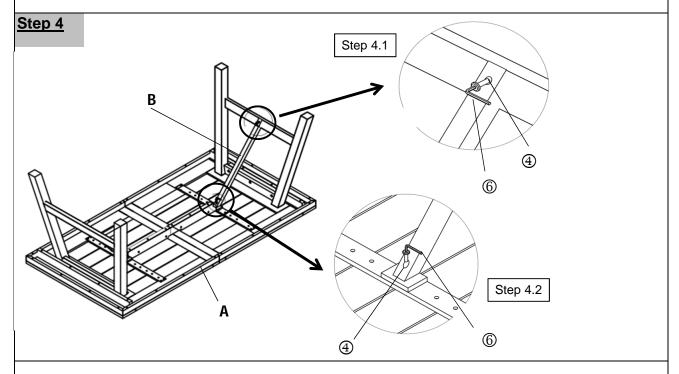
Position Leg Support Bar(B) as shown in picture above.
