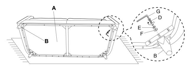
Stand loveseat up on an even surface and check that it is balanced. If there is a slight wobble, apply downward pressure in the corner where a leg is uneven. Keeping pressure in that corner, tighten all bolts. If balanced, apply downward pressure evenly in the center and tighten all bolts. Do not over-tighten beyond hole depth.
