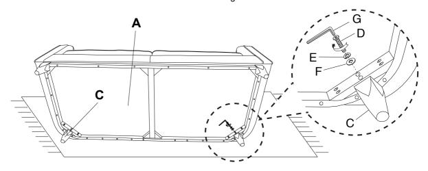
Stand loveseat up on an even surface and check that it is balanced. If there is a slight wobble, apply downward pressure in the corner where a leg is uneven. Keeping pressure in that corner, tighten all bolts. If balanced, apply downward pressure evenly in the center and tighten all bolts. Do not over-tighten beyond hole depth.
