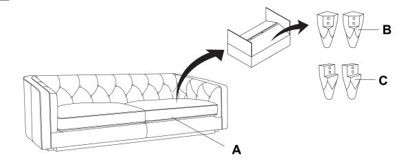
Put the Loveseat (A) on a smooth flat surface and attach Front Leg (B) to the Loveseat (A) using Bolt (D), Lock Washer (E) and Flat Washer (F) on both holes of Loveseat (A). Turn the Allen Wrench (G) in Bolt (D).
