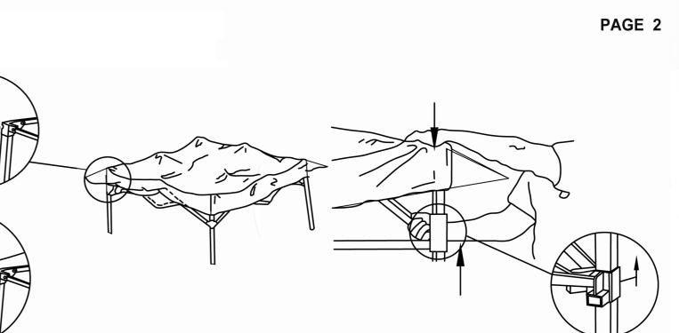
Insert Corner Rib into top corner bracket until the pin pops into place. Pull the fabric corner of canopy to wrap over the rib end. Repeat this process on the remaining corners, so the overhang is formed.
