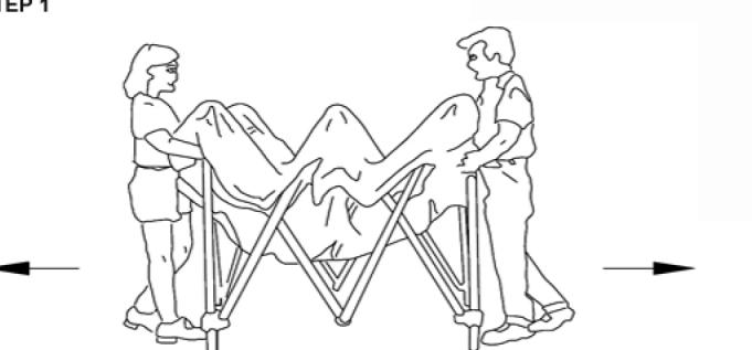
Set the gazebo frame in the center of the set-up area. Grasp the legs on one side while a partner grasps the legs on the opposite side. Working at the same time, pull out on the legs to spread the frame open as far as possible. You may need to step backward carefully to allow room to open the frame.
