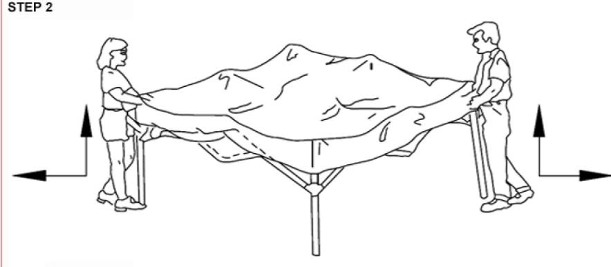
Secure each corner with the valance on the canopy, make sure the valance to fit well around the top of the leg on the frame.
