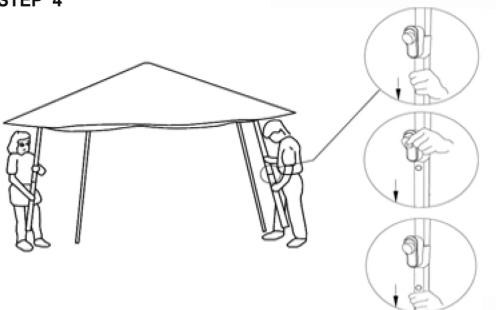
Lift the upper pole with one hand (do not press the snap button), slide out the lower pole with the other hand until it clicks into place. To rise to the second height, continue to slide the pole towards next hole by pressing the snap button, but make sure to release button immediately at the moment the pole moves, keep sliding until it clicks into place again. Repeat same process to slide up or down to reach the desired level, always make sure all 4 legs in the same level.
