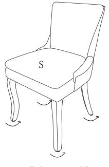
Tighten one and loosen the other, to adjust to level.
