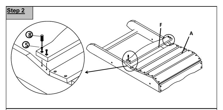
Place the Seat Panel(A) onto a clean, non-marring surface. Position KD Slat(F) onto the Seat Panel(A) and attach using 4 Screws(5) and Screwdriver(8).
