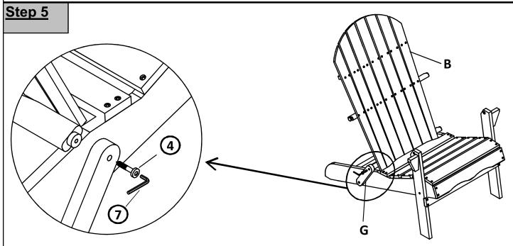
Position Backrest(B) with mortise into housing of Folding Support Bar(G). Secure Folding Support Bar(G) to Backrest(B) using Short Screw(4) with Allen Key(7).
