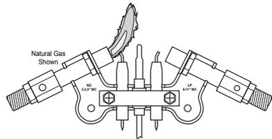
Figure 23 - Incorrect Pilot Flame Pattern (Natural Gas shown)
