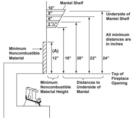
Figure 6 - Minimum Mantel Clearances Without Using Hood
