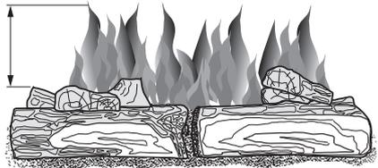
Figure 25 - Incorrect Burner Flame Pattern
