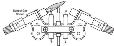
Figure 22 - Correct Pilot Flame Pattern (Natural Gas shown)
