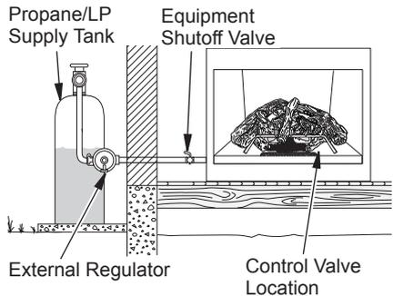
**Figure 16 - Checking Gas Joints for Propane/LP Gas**
