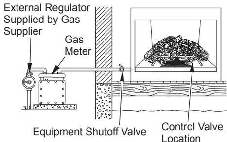
**Figure 17 - Checking Gas Joints for Natural Gas**
