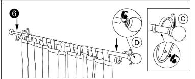
Place drapery panels (not included) onto drapery rod and extend to desired length. Hang rod on brackets. Screw finials (D) onto ends of rod and tighten set screws on brackets (C).
