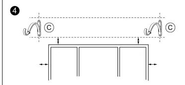
Repeat steps 2-3 for additional bracket. Use level if necessary.
