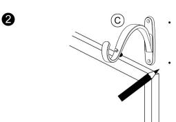
Use bracket (C) as a guide to mark location for mounting screws (A).
