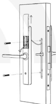
Tighten the back panel screws.
