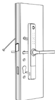
\* When you want to drill a new hole for the cable, you might need to remove the multi-point mechanism to locate a safe spot to drill.
