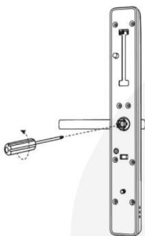
1. Loosen the screw on the Handle (Counterclockwise)
