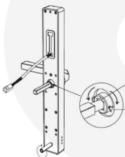
1. After fitting the spindle, insert the split pin and bend the ends with a plier.
