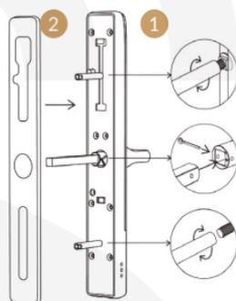
Fit the flat Head Screw to the stub and fix it into position to line up with the Door holes.
