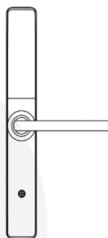
3. Rotate the handle 180 degrees and tighten back up.
