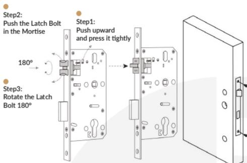
If you your existing multipoint lock is compatible with the Simplified Smart lock, skip this step. Otherwise, check if the latch direction is proper for your door. Should you change the latch direction, follow the steps in the left picture.
