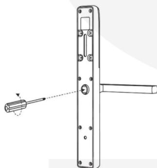
1. Loosen the screw on the Handle (Counterclockwise)
