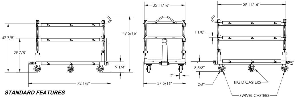
MODEL NUMBER IS AEC-3660-3-MR OVERALL WIDTH IS 37 5/16" USABLE WIDTH IS 35 11/16" OVERALL LENGTH IS 72 1/8" USABLE LENGTH IS 59 11/16" OVERALL HEIGHT IS 49 5/16" FOUR MOLD ON RUBBER Ø6" X 2" SWIVEL CASTERS TWO MOLD ON RUBBER Ø6" X 2" RIGID CASTERS
