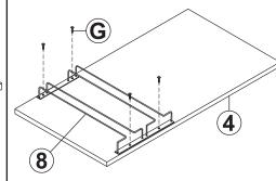
STEP 3 **9**: 2 **10**: 2 **K**: 4 Cam Screw must align with Cam Lock hole **Proper Cam Screw Installation**
