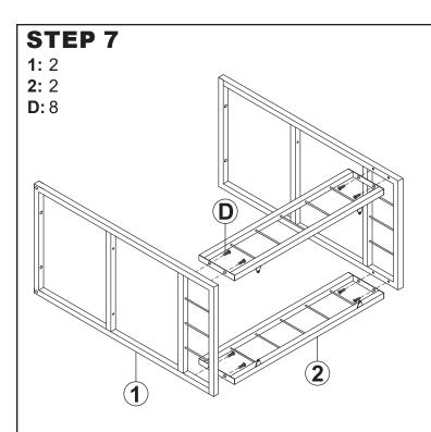
Identify the metal tabs on Bottom Rails (2). Ensure the rails are installed with the tabs on the bottom and facing the inside of the cart.
