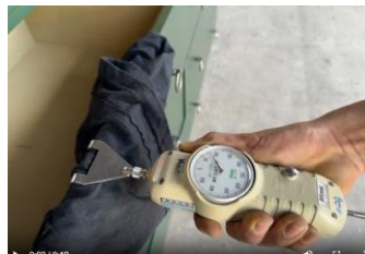
Apply a 10 lbf (44 N) horizontal force at the highest-level drawer, not tip over
