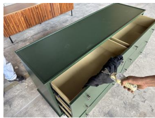
Apply a 10 lbf (44 N) horizontal force at the highest-level drawer, not tip over
