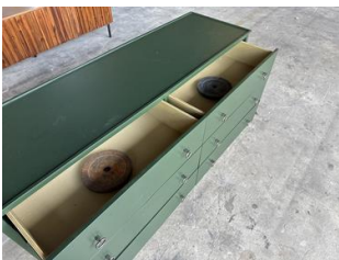
10kg weigh each drawer, not tip over
