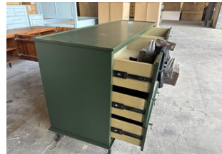
60lbs at the highest-level drawer, not tip over
