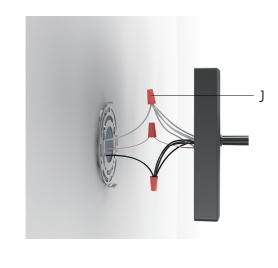
Also, we have pointed screws as well as expansions for when you don't have a pre-installed base in your home. Mounting plate can be mounted directly to the wall using pointed screws and expansion.
