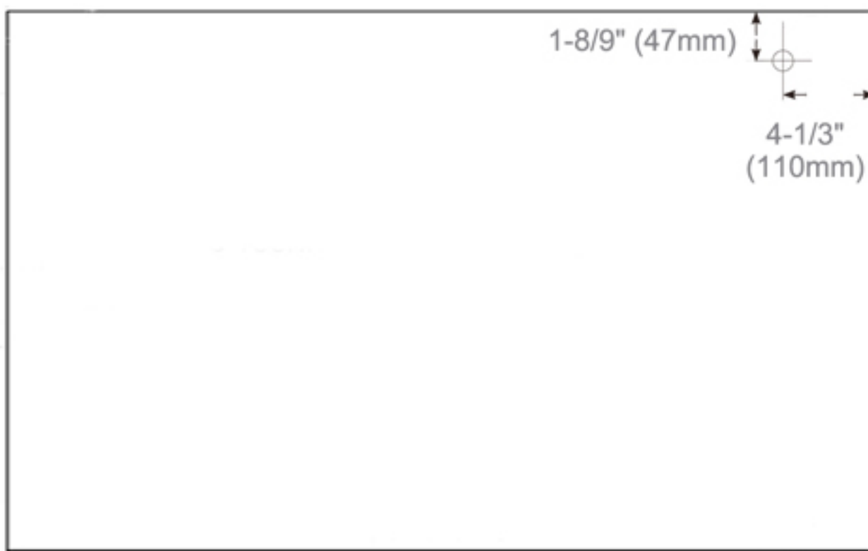
Back of Cabinet - Wire Access Location
