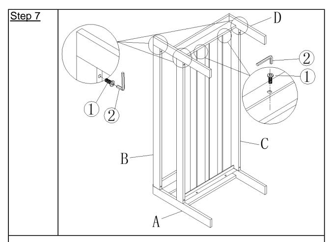
**7.1**) Attach the Leg Support Bar(D) to Back Support Bar(B) and Seat Panel(C) using Bolts(①) with Allen Key(②) as shown above.
