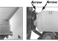
**8.** Push **EXPRESS PUMP**<sup>®</sup> firmly into valve (d). Do not force. Twist pump to lock into place (e). Turn on switch to begin inflating (f).
