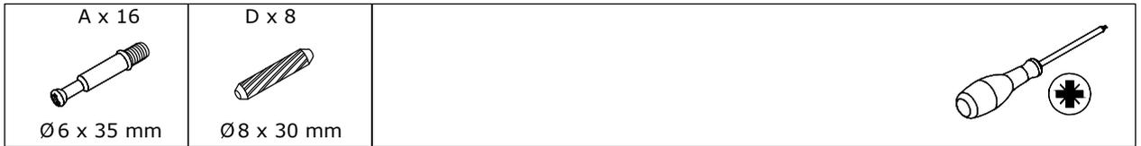
Cam Bolt (A) to plate 5 with across screwdriver, as shown.
