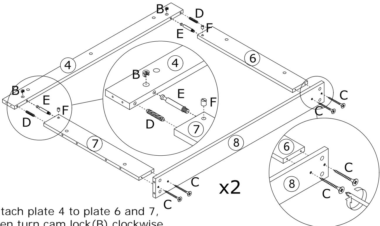
Attach plate 4 to plate 6 and 7, then turn cam lock(B) clockwise to tighten as shown.
