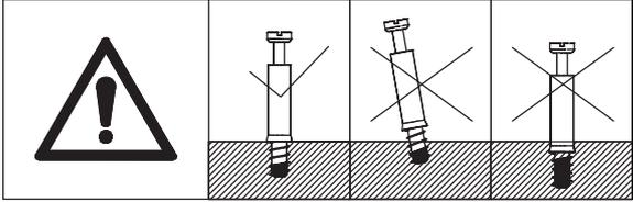
Insert quickfit screw(A) into No.12 and No.13 plate with a screwdriver as shown.
