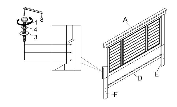
STEP 2 Assemble the HB crossbar (D) to HB legs (E & F) by using Allen Key (8)with hardware 1,3, and 4. \*TIGHTEN ALL THE BOLTS BY USING ALLEN KEY (8)
