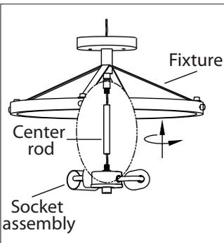
1. Screw the center rod and socket assembly to the fixture.
