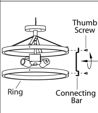
2. Remove the thumb screws that are already on the fixture and the ring. Install the ring to the fixture with the connecting bars by tightening the thumb screws.
