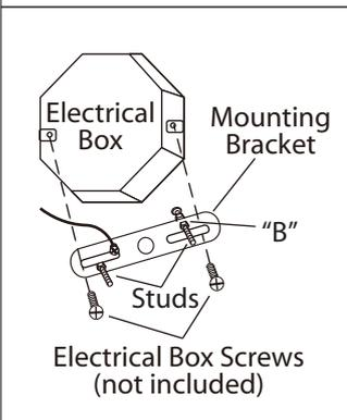
3. Loosen "B". Adjust stud to desired length and lock in place with "B". Mount the mounting bracket to electrical box using electrical box screws (not included). Make sure the studs on the mounting bracket are facing out from the electrical box.
