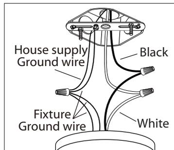
4. Connect the ground wires (bare copper or green) from your fixture to the ground wire (bare copper or green) or ground screw in the electrical box. Connect the black wire from the fixture to the black wire in the electrical box and connect the white wire from the fixture to the white wire in the electrical box.
