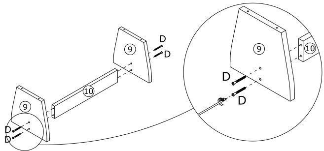
Secure panel 11 to panel 9 using screws (D) as shown.
