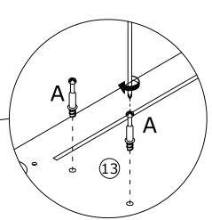
Connect panel 13 to panels 14 and 15 as shown and add cam lock (B) and tighten by turning clockwise.
