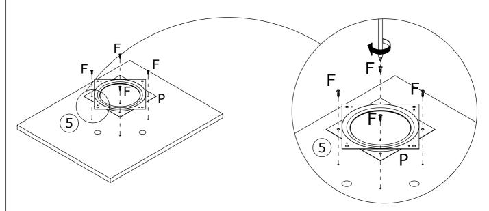
Use screws (F) to secure part (P) to panel 2 as shown.
