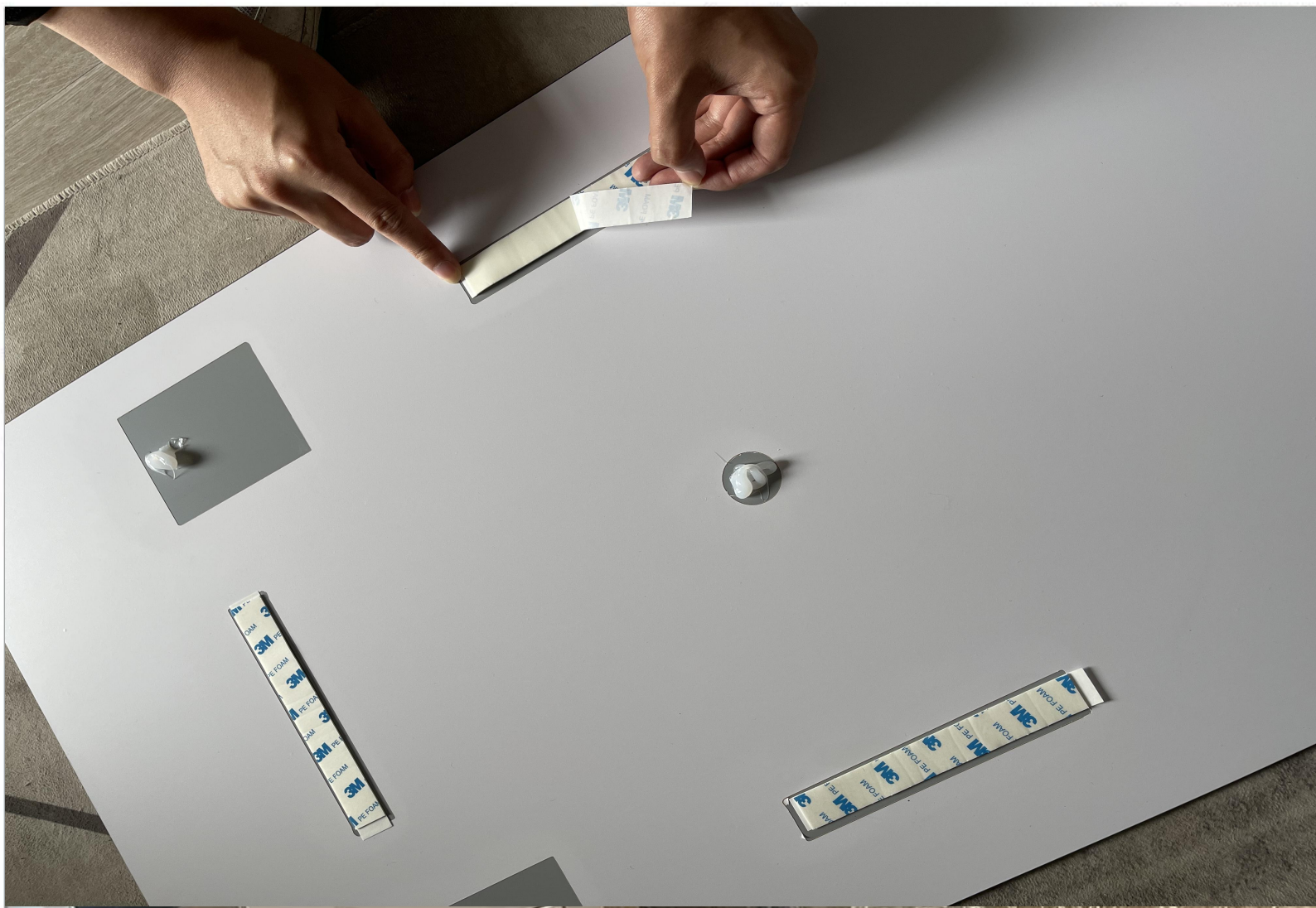
5.Tear off the top layer of double-sided tape.
