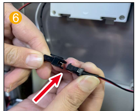
Dock the sockets of the top lamp post and the display screen
