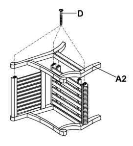
Attach left side frame (A2) to the assembly from step 1, insert 2" bolts (D).
