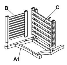
Attach back support (B) and seat (C) into right side frame (A1)
