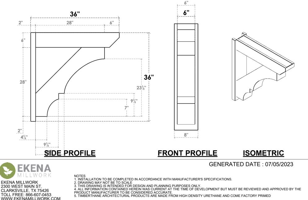
5. TIMBERTHANE ARCHITECTURAL PRODUCTS ARE MADE FROM HIGH DENSITY URETHANE AND COME FACTORY PRIMED
