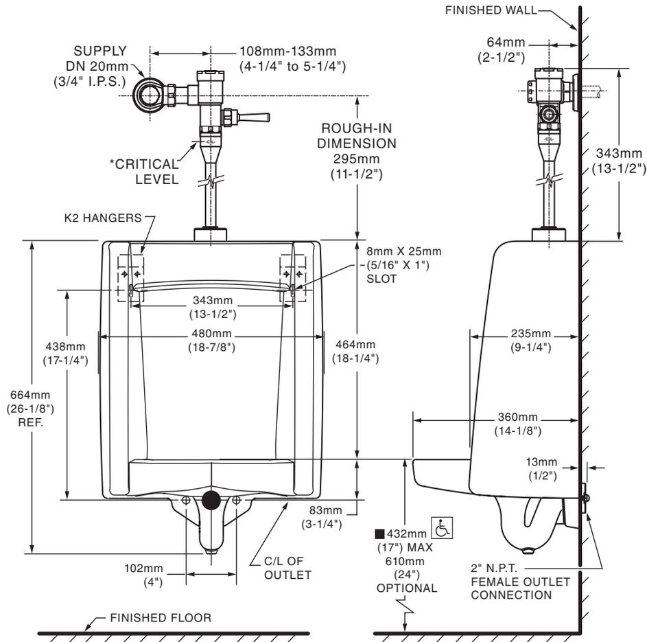
\*Note: The Critical Line (-C-L) on Vacuum Breaker must typically be a minimum of 6" (152mm) above fixture. Consult Codes for details.
