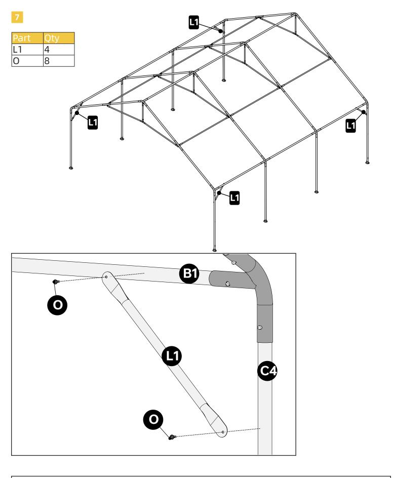
You will need a power tool drive O into the tubes. Notice that you will not find predrilled holes on the tubes for O. Do not worry too much about pinpointing the exact location for L1. The location contributes little to the stability.
