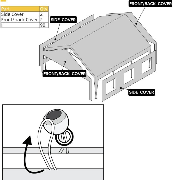
Use bungee cord, Part No. I, to fasten the covers onto the tubes.
