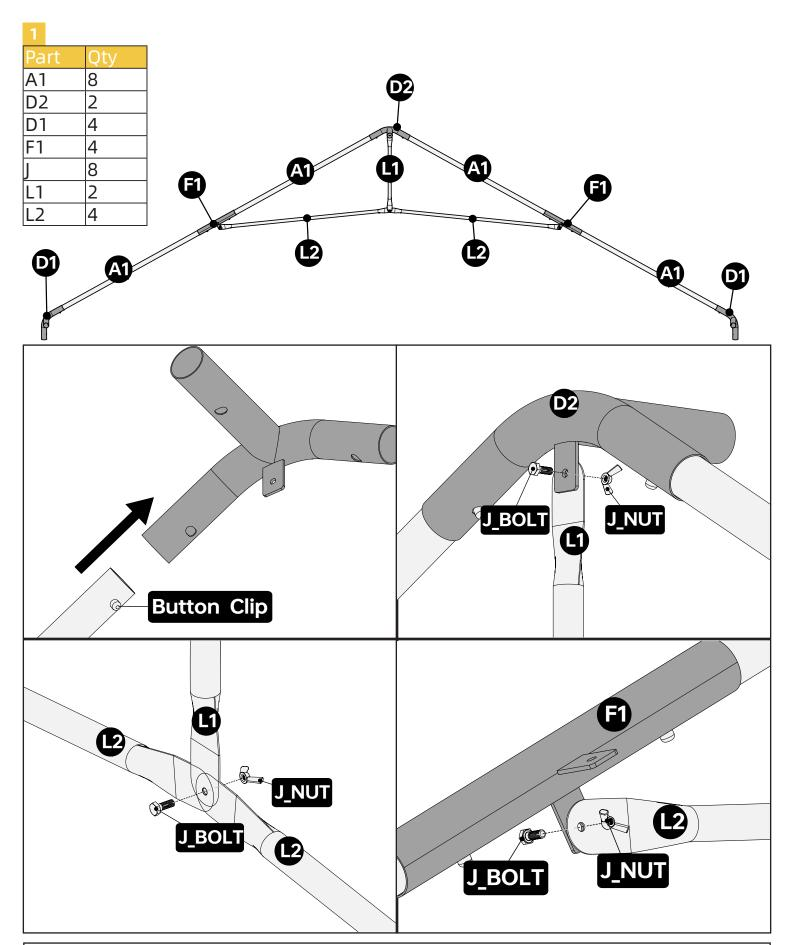
For this product, tubes and joints are connected using button clips. Button clips are already inserted inside tubes. When connecting, press the button clip and insert one tube into the joint. Forcing the tubes in might also work but you are risking damaging the Clip.
