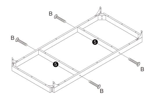
Friendly Tips: Do not fully tighten all screws until assembly is completed.
