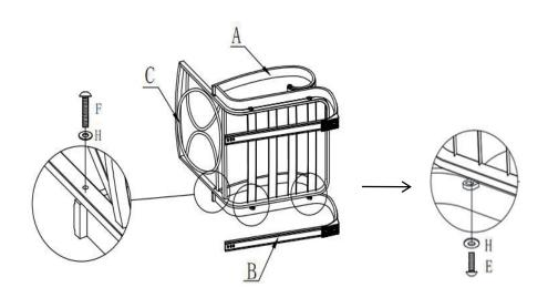
A. ATTACH REAR LEG CONNECTOR (D) TO CHAIR FRAME (C) ASSEMBLY AND (A) USING LEG LEVELER (G), FLAT WASHER (H) AND BOLT (E) USING ALLEN WRENCH (I). DO NOT TIGHTEN COMPLETELY.
