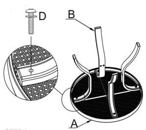
A. ATTACH LEG CONNECTOR (C) TO LEGS (B) WITH FLAT WASHERS AND BOLTS (D) USING ALLEN WRENCH (E). DO NOT TIGHTEN COMPLETELY.
