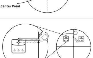
Measure the distance between the center point of the clips and write down the result.
