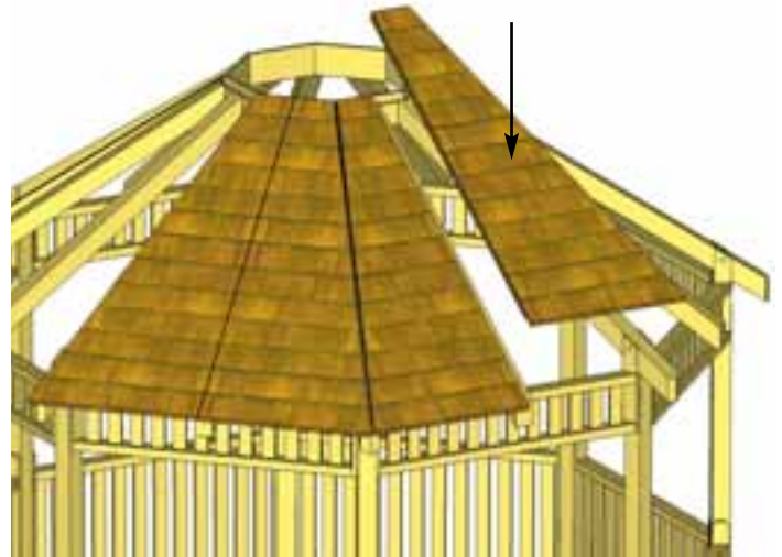
71. Position and attach as per Step 66 - 67. Use 2 - 3" screws in Corner Rafter and Mid Rafter through bottom row of shingles. Lift and position 2nd Right Side Roof Panel on Center and Corner Rafter.
