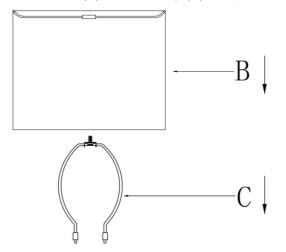
Step 5. Secure the shade (B) by turning the finial (A) onto the harp top clockwise until tight.
