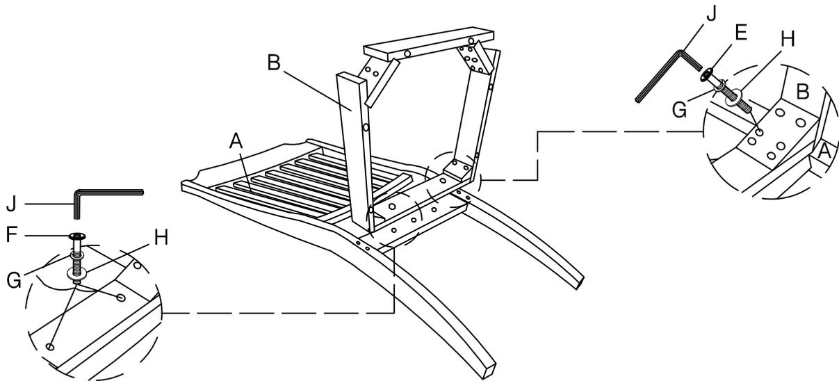
Take the Allen Wrench, and turn the bolts until the legs are secure.
