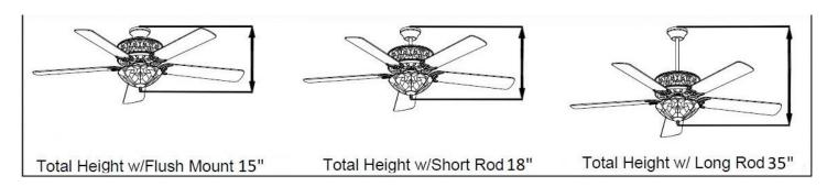
You may install your ceiling fan as a flush mount, or you may use the provided down rod(s). Measure your room height before installing the fan and consider the different installation height options indicated in the above diagram.
