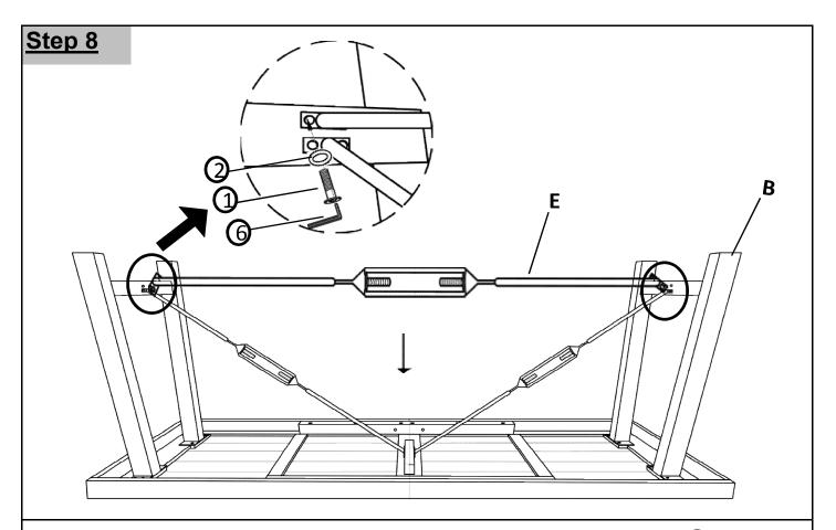
Attach the Bottom Turnbuckle Set(E) to Iron Legs(B) using Short Bolt(1) and Washer(2) with Allen Key(6).
