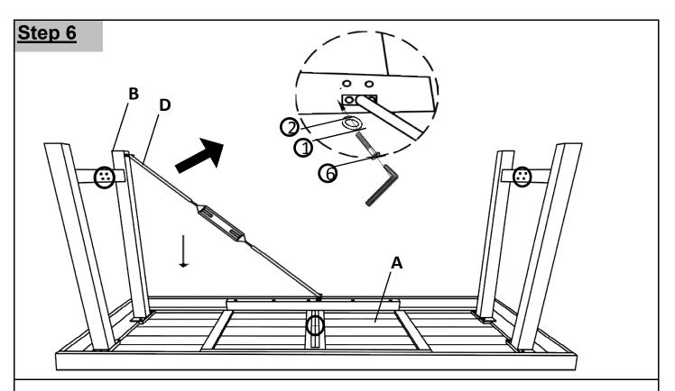
Place Side Turnbuckle Set(D) between housing of Table Top(A) and Iron Leg(B). Attach Side Turnbuckle Set(D) to Iron Leg(B) using Short Bolt( $\widehat{1}$ ) and Washer( $\widehat{2}$ ) with Allen Key( $\widehat{6}$ )
