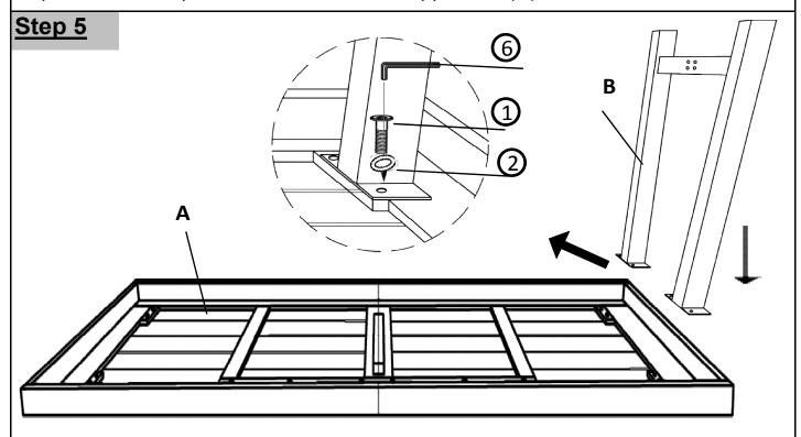
Attach Iron Leg(B) to Table Top(A) using Short Bolt((1)) and Washer((2)) with Allen Key((6)).
