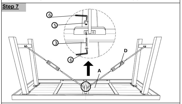
Affix Side Turnbuckle Set(D) to Table Top(A) using Long Bolt( $\widehat{3}$ ) and Sleeve Nut( $\widehat{5}$ ) with Allen Key( $\widehat{6}$ ).
