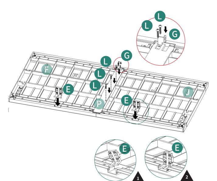
For easier installation, part E should tilt to the one side, then to the other.
