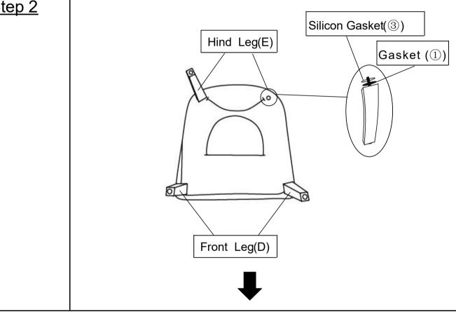
Install the first Front leg(D) onto the Chair(B) by placing one Gasket(1) onto the threaded stem. Insert the threaded stem of the Front Leg(D) into one of the front mounting positions of the Chair(B), then tighten by turning the Leg clockwise until it is completely secure.
