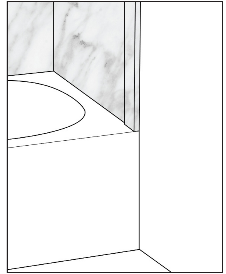
Vertical trims installed to top of tub
