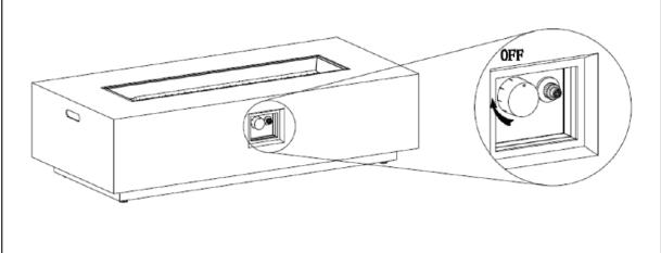
1. Check that the Control Knob (15) for the gas supply system is turned to the "OFF" position before starting any assembly.
