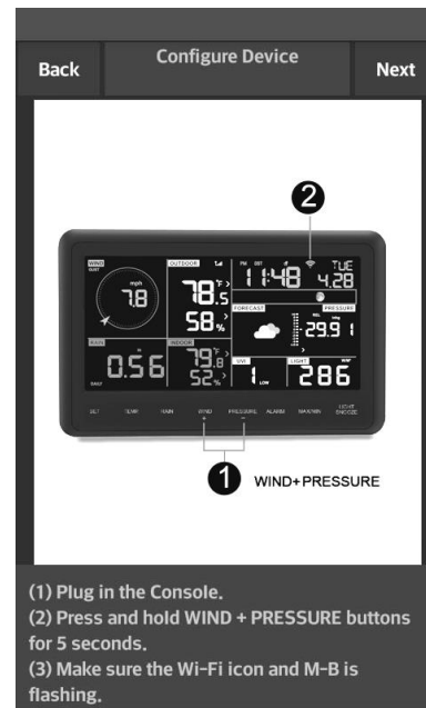
(c) Make sure the Wi-Fi icon is flashing rapidly. If not, press and hold the WIND+ and PRESSURE- buttons for four seconds.
