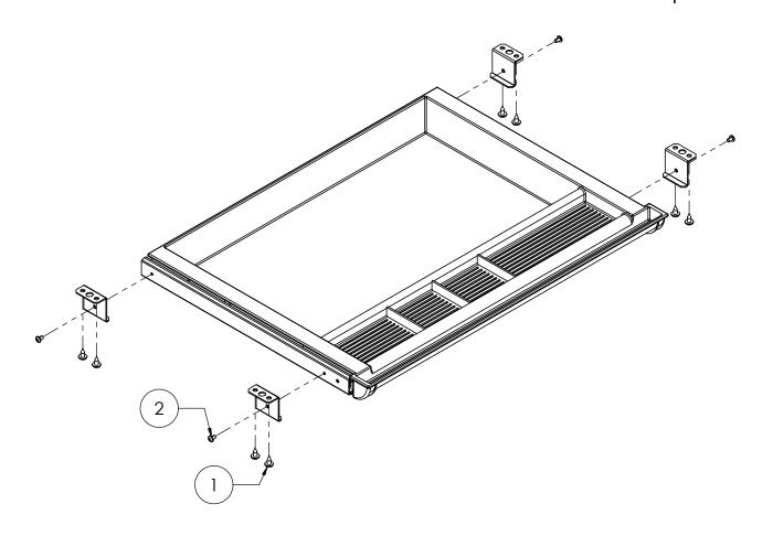
Attach the brackets and mark and drill eight 5/64" pilot holes 1/2" deep. Put one screw <u>1</u> in each bracket and fully tighten. Operate the drawer. If it is binding, loosen the screws and adjust the drawer until it is not binding. Tighten the screws and drive in four more screws.
