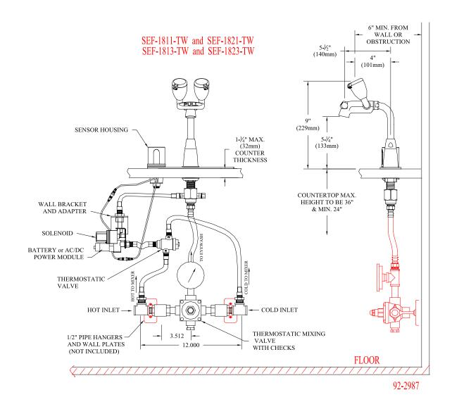
SEF-1811-TW -4" Sensorflow, eyewash faucet, TMV, battery and Thermostatic Valve for Eyewash -4" Sensorflow, eyewash faucet, TMV, AC/DC and Thermostatic Valve for Eyewash SEF-1813-TW -8" Sensorflow, eyewash faucet, TMV, battery and Thermostatic Valve for Eyewash SEF-1823-TW -8" Sensorflow, eyewash faucet, TMV, AC/DC and Thermostatic Valve for Eyewash
