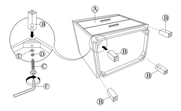
Insert Leg (B) at position as shown and tighten with JCBC Screw (C), Spring Washer (D) & Flat Washer (E) by using Allen key (F)  $\,$
