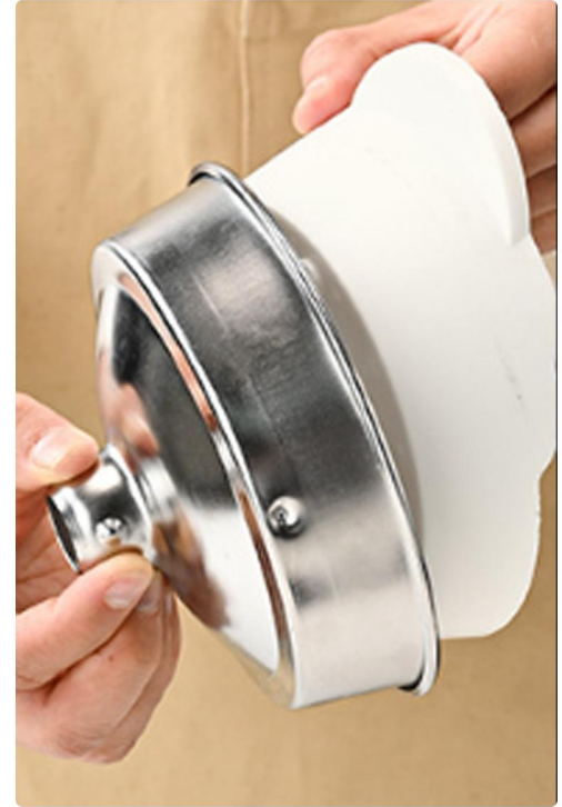
③ Pinch the chuck buckle to separate the pressure plate and funnel
