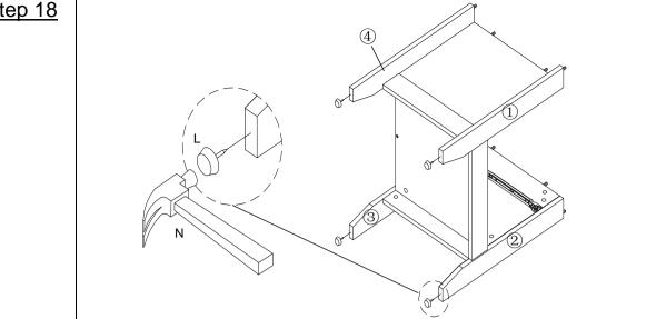
**18.1)** Attach the Leg Stud (L) to the Bottom of Left Front Leg (1), Right Front Leg (2), Right Rear Leg (3), and Left Rear Leg (4) using hammer (N).
