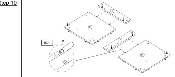
**10.1)** Apply Glue (K) into the dowel mounting positions on Horizontal Panel (7). Attach Left Side Panel (5) to Horizontal Panel (7). Repeat the same steps to Assemble Right Side Panel (6) to Horizontal Panel (7).
