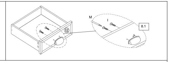
8.1) Attach Handle (J) to Drawer Front (12) using Truss Head Screws M4 x 12mm (I) and screwdriver (M).
