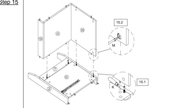
**15.1)** Apply Glue (K) into the dowel mounting positions on Right Front Leg (2), Horizontal Panel (7) and Right Side Panel (6).
