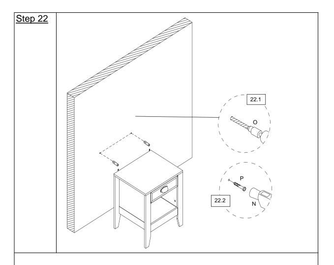
**22.1)** Drill two holes on the wall at the same height as the Webbing on the Nightstand using a Power Drill (O).
