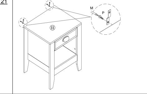
**21.1)** Attach the Webbing (P) to the pre-holes on the back side of Top Panel 1 using screws M3.5 x 12mm (P) with screwdriver (M).
