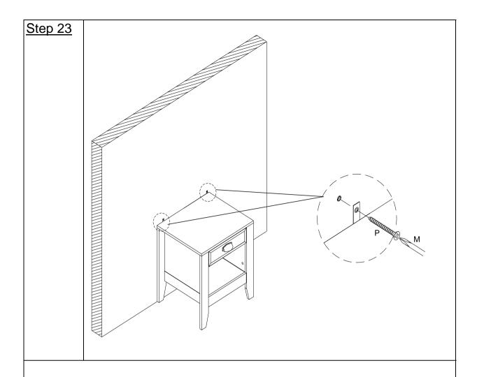
Move the Nightstand to the wall, and secure the Nightstand using Screws M4.5 x 38mm (P) and screwdriver (M).
