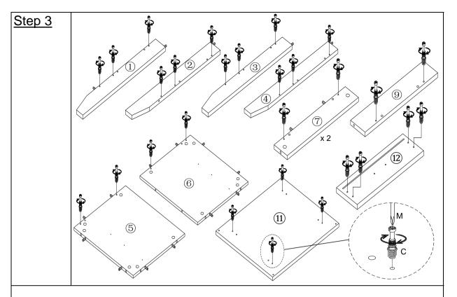
**3.1)** Insert Cam Bolts (C) into the the mounting positions on Left Front Leg ①, Right Front Leg ②, Right Rear Leg ③, Left Rear Leg ④, Left Side Panel ⑤, Right Side Panel ⑥, Horizontal Panel ⑦, Support Panel ⑨, Top Panel ⑪ and Drawer Front ⑫ with screwdriver (M).
