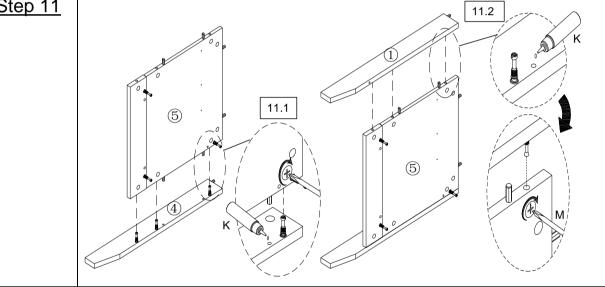
**11.1)** Apply Glue (K) into the dowel mounting positions on Left Rear Leg (4). Attach Left Side Panel (5) to Left Rear Leg (4).
