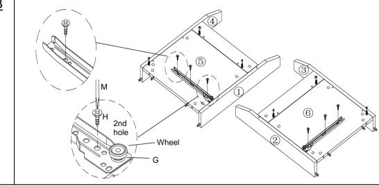
**13.1)** Attach the Left Silde (G) to Left Side Panel (5) and the Right Slide (G) to Right Side Panel (6) using Screws M4 x 12 (H) and screwdriver (M).
