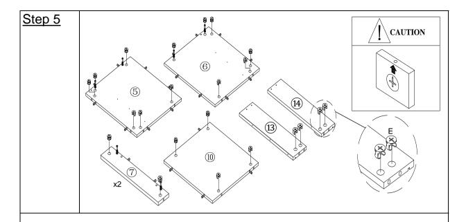
**5.1)** Insert Cam Locks (E) into the mounting positions on Left Side Panel (5), Right Side Panel (6), Horizontal Panel (7), Back Panel (10), Left Drawer Side Panel (13) and Right Drawer Side Panel (14).
