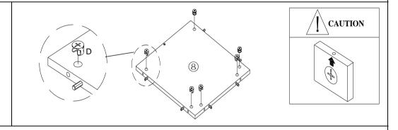
**4.1)** Insert Cam Locks (D) into the mounting positions on Bottom Panel (8).
