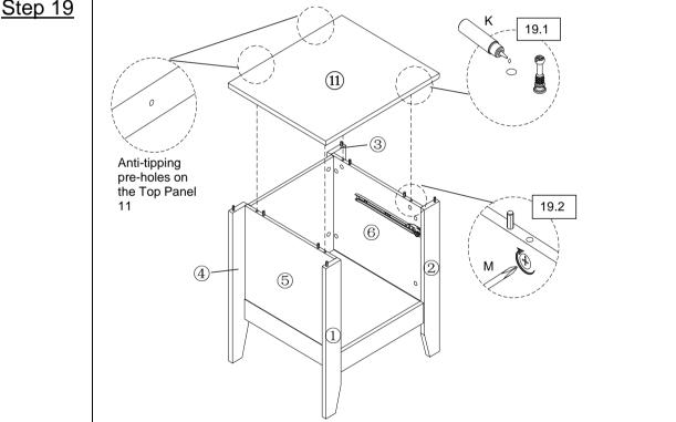
**19.1)** Apply Glue (K) into the dowel mounting positions on Top Panel (1).
