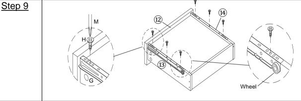
9.1) Attach the Left Slide (G) onto Left Drawer Side Panel (3) and Right Slide (G) to Right Drawer Side Panel (4) using Screws M4 x 12mm (H) and screwdriver (M).
