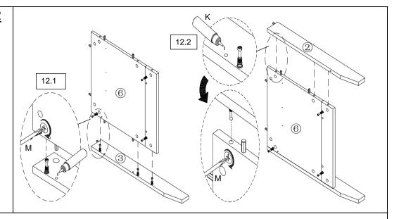
**12.1)** Apply Glue (K) into the dowel mounting positions on Right Rear Leg ③. Attach Right Side Panel ⑥ to Right Rear Leg ③.
