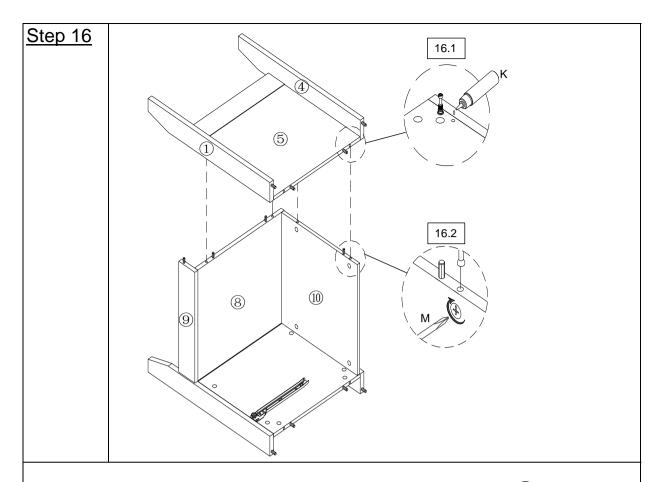
**16.1)** Apply Glue (K) into the dowel mounting positions on Left Front Leg 1, Horizontal Panel 7 and Left Side Panel 5.
