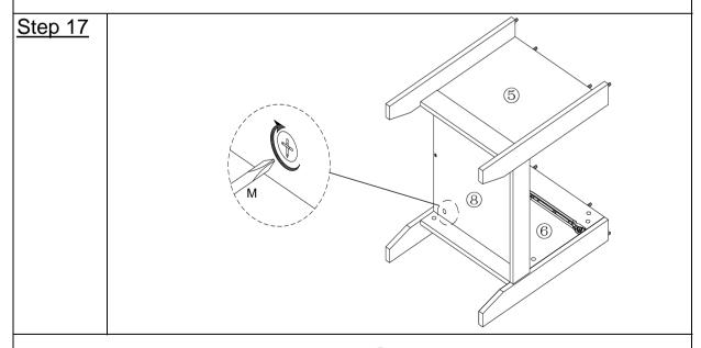
**17.1)** Turn the Cam Locks (D) on Bottom Panel (8) clockwise with screwdriver (M) until they lock into place.
