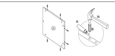
**2.1)** Apply Glue (K), and insert Wood Dowels M8x25mm (B) into the mounting positions on the
