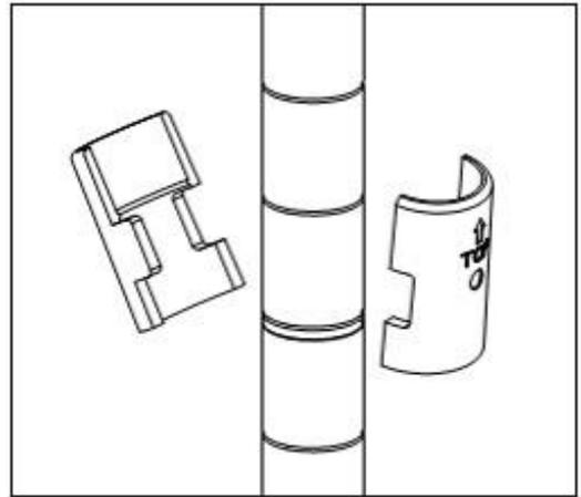
*Note: There will be a very small gap in-between two locked SLIP SLEEVES (E)—this is normal.*
